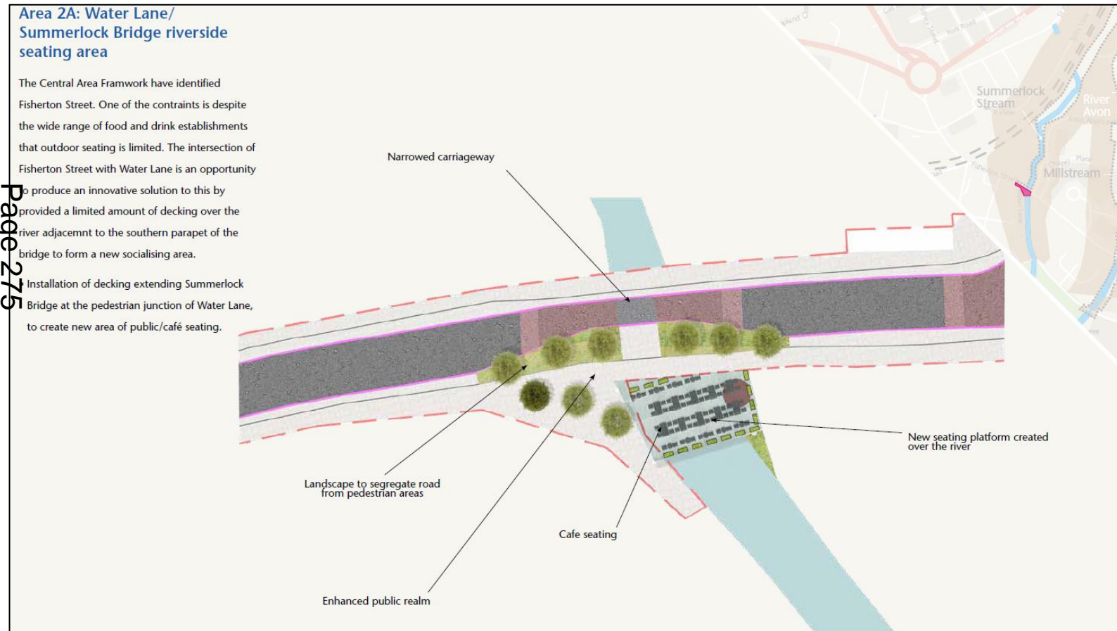
Figure 2.1: Phase 2A – Summerlock Bridge
